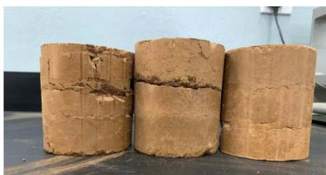
Figure 1. Preparing the 40 samples for testing compressive strength (Authors).
