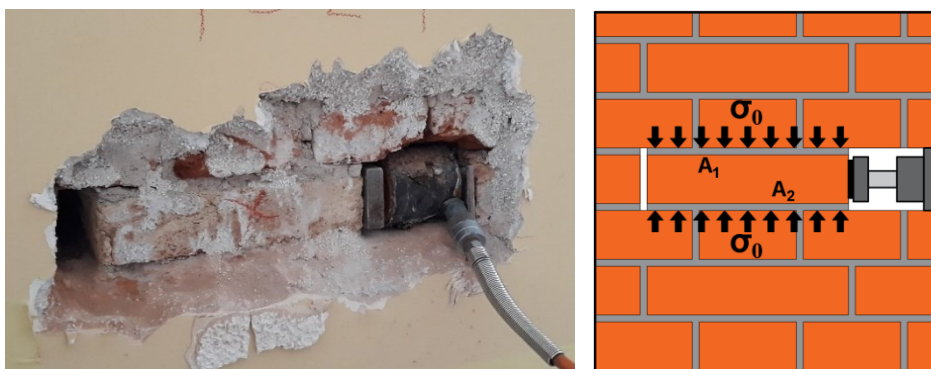
Figure 4. Shear test setup
