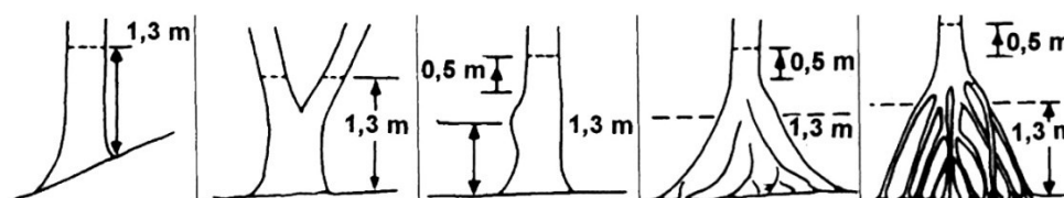
Figure 2. Measurement of tree diameter at a height of 1.3 meters (Hairiah, 2001).
