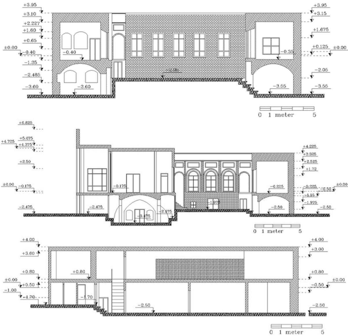
Figure 6. The Designed Sections of the Museum of Poets: (from above to below) The Designed A-A Section of the Qajar Building of the Museum of Poets, The Designed B-B Section of the Qajar Building of the Museum of Poets, The Designed C-C Section of the Pahlavi Building of the Museum of Poets (Asbagh, 2011, PP. 145, 146).
