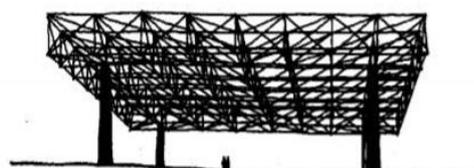
**Figure 8.** Space frame system(Allen,2005).
