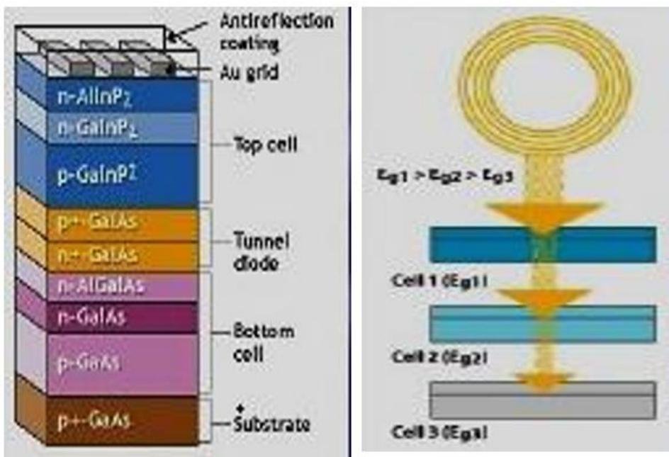
Figure 16: thin film solar cell junctions structures source developed by author
