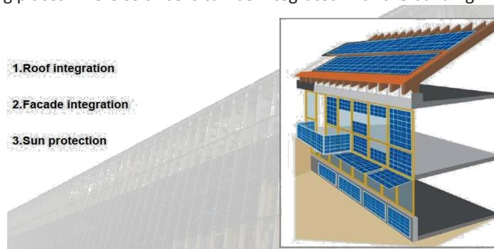
**Figure 6.** integrating solar cells with building , ( shaybani, 2016)
