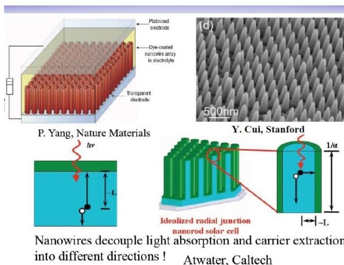
Nanowires decouple light absorption and carrier extraction into different directions ! Atwater, Caltech
