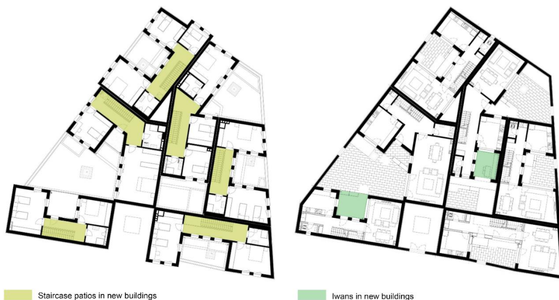
Figure 8: Iwans and staircase patios in the houses
