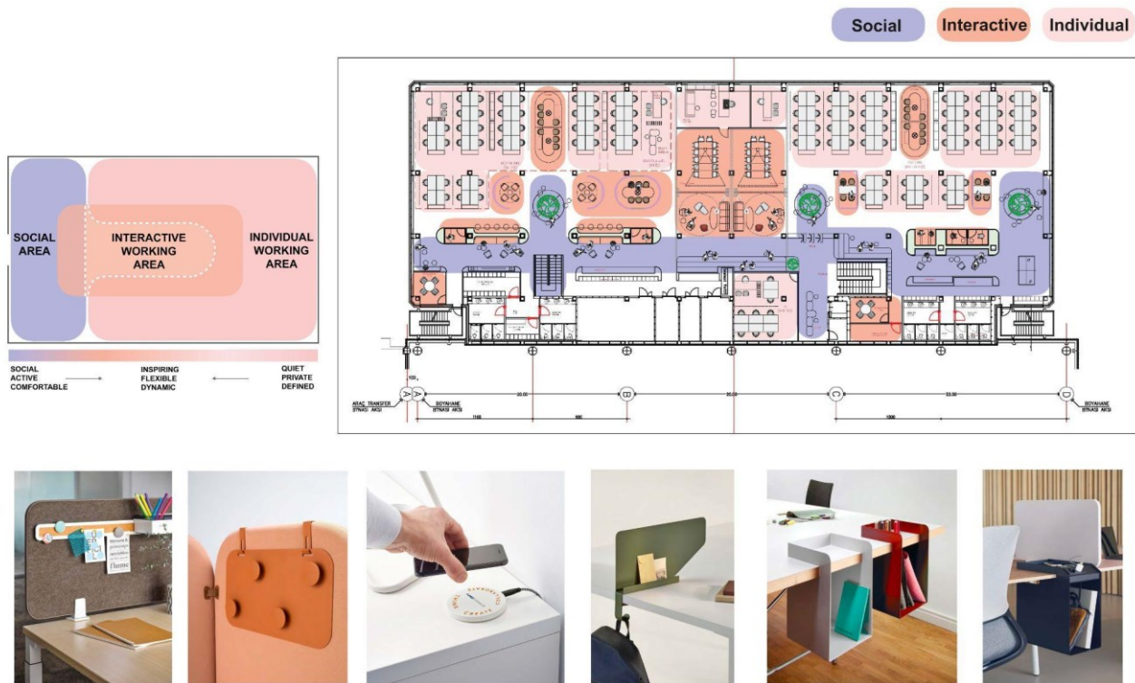
Figure 3. Agile working solutions and strategic organization of social, interactive, and individual areas (by the design team I-AM)
