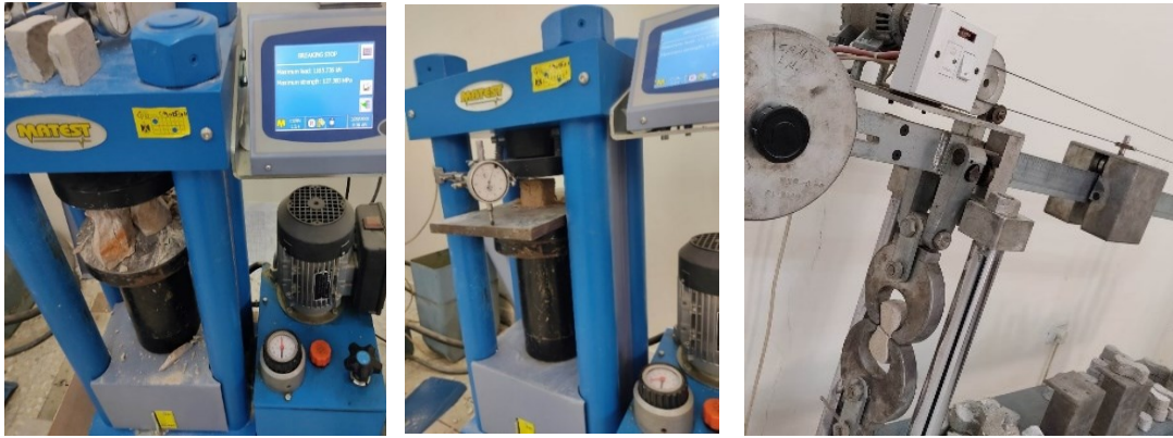
Figure 3: Compressive strength of (10*10*10) stone, Compressive strength & Tensile strength of lime mortar and lime mixtures.
