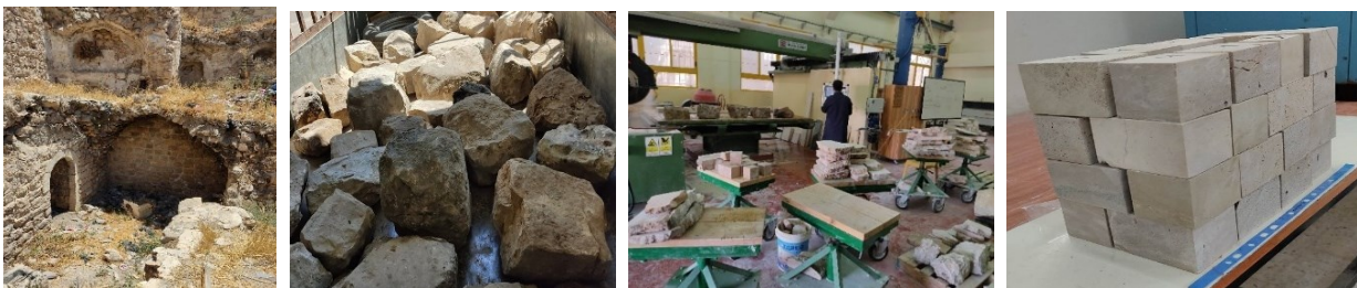
Figure 2: source location of historical stone & stage of preparing it to cut it into suitable pieces by CNC for experiments.
