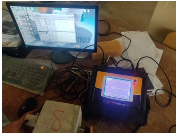
Figure 6. Pre-cracking protocol and sonic time wave velocity measurements
