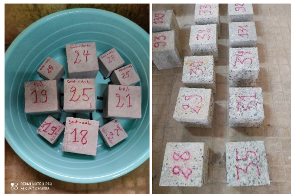
Figure 7. Sulfuric attack testing
