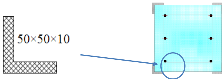
Figure 5: Retrofitting details with steel caging
