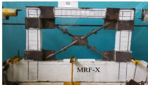
Figure 2. Retrofitting of RC frames with steel bracing [31]
