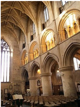
Figure 13. Ribbed vault showing the triforium and the clerestory windows.
