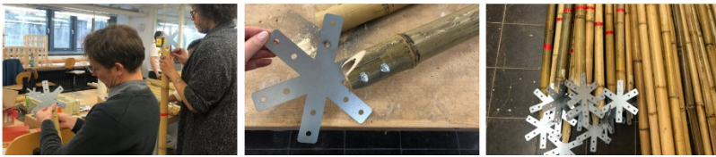
Figure 7: Adding a connector to the red marked bamboos. Own Source, Abanoz, B., 2025.
