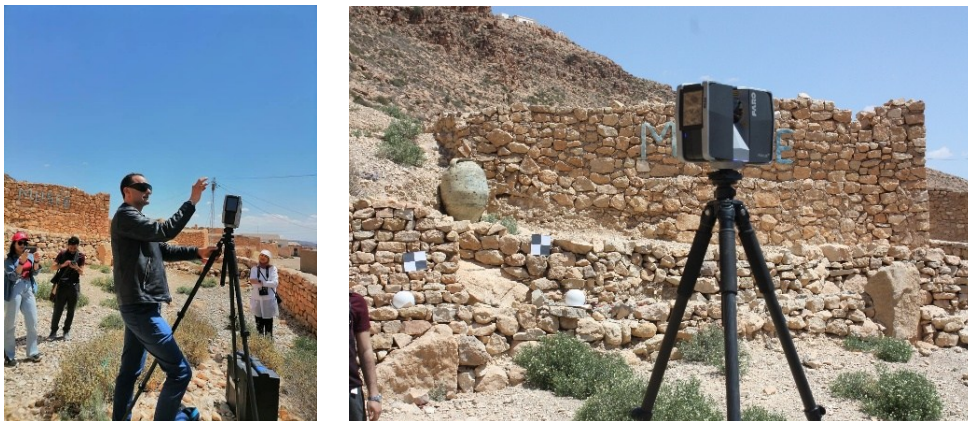
Figure 4. 3D Scan Campaign of the Studied Oil Mill in Toujen and the 3D Laser Scanner Used (Source: Authors).
