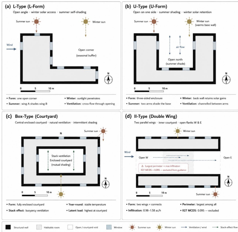
Figure 1. Four residential plan morphologies studied with passive thermal strategy annotation: L-Form (open corner), U-Form (open south), Courtyard (box) (central courtyard), and II-Form (double wing). All configurations are two storeys, 4.0 m floor height, with a courtyard facing glazing fraction of 30%.
