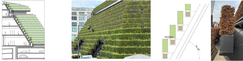
Figure 7. Kö-Bogen II building structure and shell system (a. (Kaltenbach, 2020), b. Sirel (2025), c. d. Anderson (2023), e. (Schüller-Plan, n.d.), f. (BauNetz Wissen, n.d.), g. i. Sirel (2025), h. (Landeshauptstadt Düsseldorf, n.d.)
