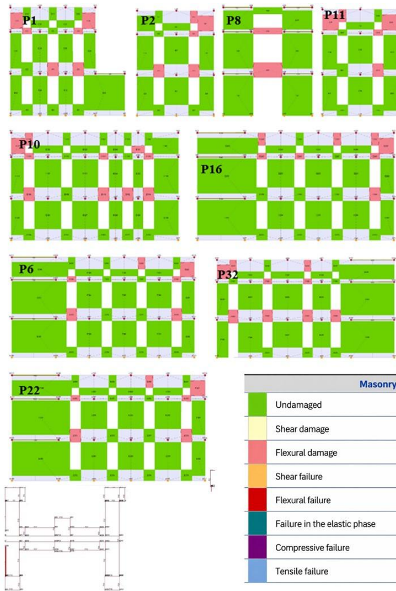
Figure 12. Wall damage state of El Feth Highschool – Pushover analysis (positive X-direction). Source: (Developed by authors).
