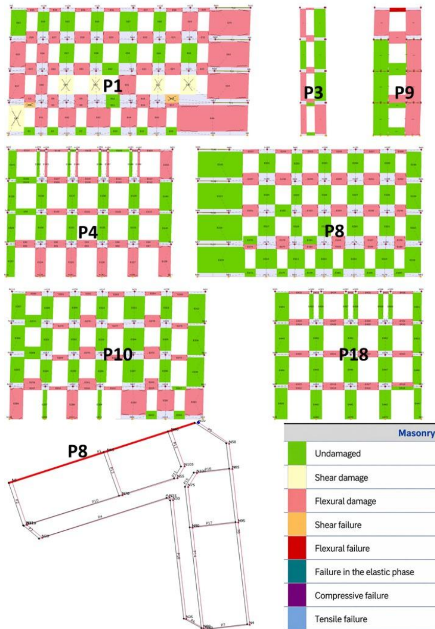
Figure 8. Wall damage state of Okba Highschool – Pushover analysis (positive X-direction). Source: (Developed by authors).
