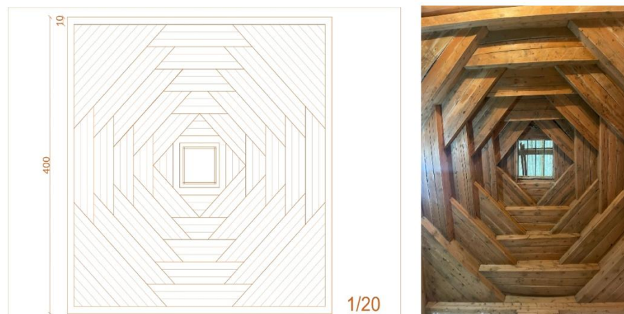
Figure 6. From left to right: plan drawing of the kirman ceiling and the kirman ceiling (Personal Archive of Seval Akbulut, 2026).
